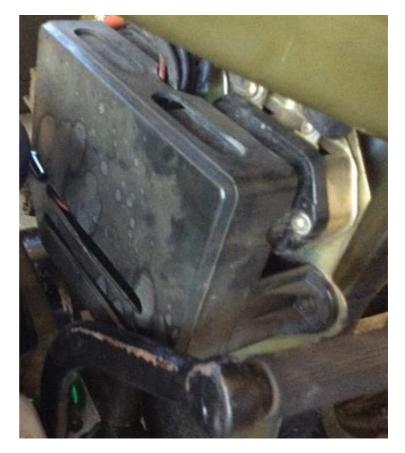
Part A, Point 8: Looking across the airbox towards the rear of the bike, there are three items on the metal electrical parts board. The upper left black box is the starter relay (often termed the "solenoid") which must remain where it is. The upper right black box is the voltage regulator (occasionally termed the "adjuster") which will be removed. The lower central item is the rectifier (often termed the "diode board") which will also be removed.
