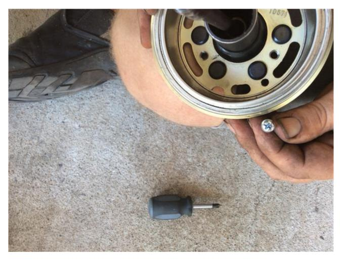
This photo shows the damage which resulted when we added washers from the old screws which mounted the old stator under the heads of the new smaller screws which were to mount the new stator.
