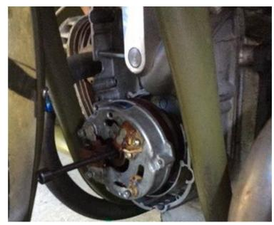
**Part A, Point 5, sub-point 2:** Remove the rotor. The front of the engine should now look like this:
