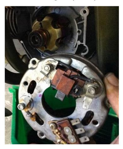
Part A, point 5, sub-point 1: Remove the Allen-headed rotor bolt which fastens the rotor to the crankshaft. This needs an 8mm Allen-key. Note that this bolt needs to be unscrewed three times during its removal. (As you may note from the pictures, I actually did this before removing the stator — exact order is often not something to get pedantic about!) Keep this bolt as you will need it again in Part B.
