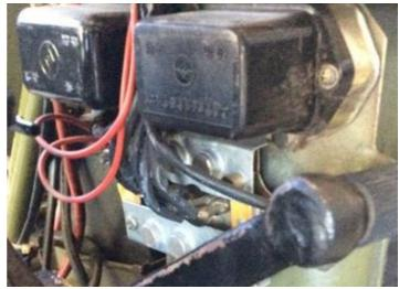
In this photo we see a better view of the voltage regulator above and the diode-bridge rectifier (often termed "diode board") below which must both be removed.
