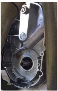
**Part A, Point 6:** Remove air-cleaner by unscrewing two grub screws; one on each side. Unfortunately I left this in place until later on, as you can see in some of the photos, and it kept getting in the road of the other work I was attempting to do. It is only thirty seconds to do, so learn from my mistake and do it now!
